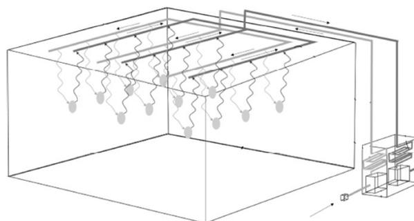
Figure 3: Schematic view of a preferred implementation mode of the communal air disinfection system. The arrows indicate the direction of the air flow
