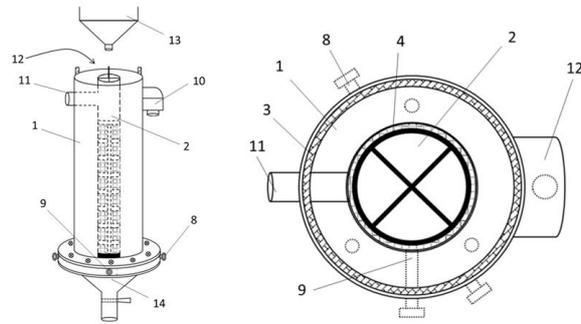
Figure 1: schematic view -front and top, respectively- of the electrochemical reactor in concentric cylindrical electrode configuration.
