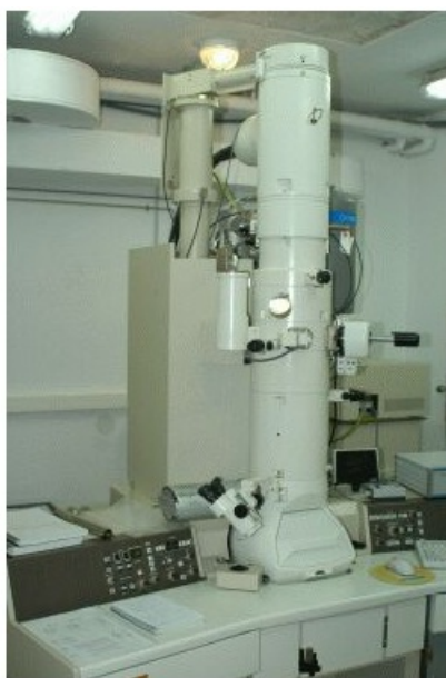
Figure 2. Transmission electron microscope (JEOL, model JEM-2010) of the Technical Research Services of the University of Alicante.
