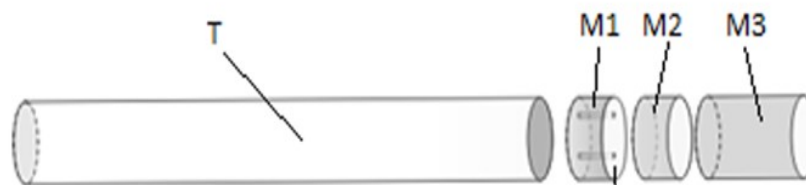
Figure 1: tobacco column (T) and combined filter formed by: the primary membrane (M1), the intermediate membrane (M2) and the outer membrane (M3).
