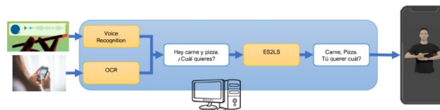
Figure 2: Diagram of the functionality corresponding to the generation of the signing by means of a virtual avatar from text or audio entered by a user.
