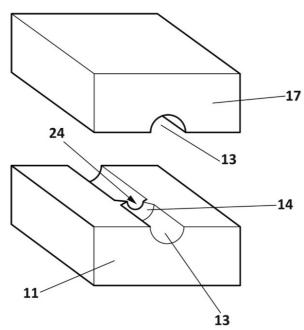
Figure 5: Perspective view of a portion of the half-moulds showing one of the cores extending from the base of the channel.
