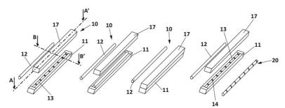
Figure 2: perspective views of operations carried out on a fibrous bar where the semi-mould bodies are longitudinal and directed in opposite directions towards the fibrous bar.
