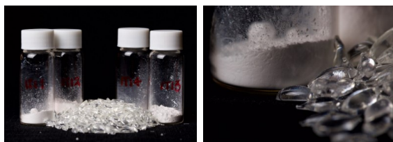
Image 1 and 2: vials with the new catalysts designed at the UA, and sample of plastic transformed into hydrocarbons.
