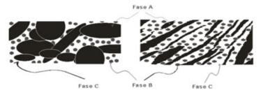
Although the three phases must have good thermal properties, it is phase A (graphite flakes) the one responsible for the properties of this innovative material. Phase B acts as a separator (or spacer materials) of the layers of phase A enabling the infiltration of phase C which consolidates the preform. The amount of alloy employed should be enough to fill the preform pores in order to obtain a composite material with the lower porosity possible.
