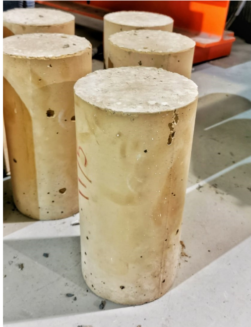
Ecological concrete test tube for compressive strength tests.
