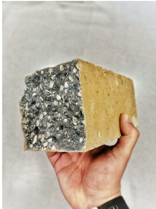
Cross-section of ecological concrete specimen after flexural breakage.
