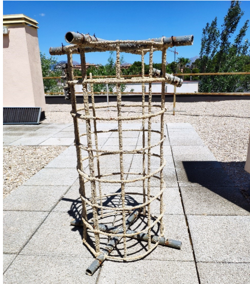
Figure 8: metal structure with the calcareous coating obtained by electrolysis.
