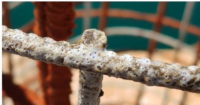
Figure 1: aspect of the calcareous coating at the end of the electrolysis phase.
