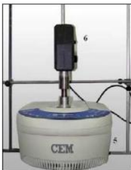
Figure 2. Microwaves and ultrasounds coupled system to irradiate simultaneously, consecutively or alternatively, solid or liquid samples, with both kinds of energy. (5) Microwaves system; (6) Ultrasounds system.
