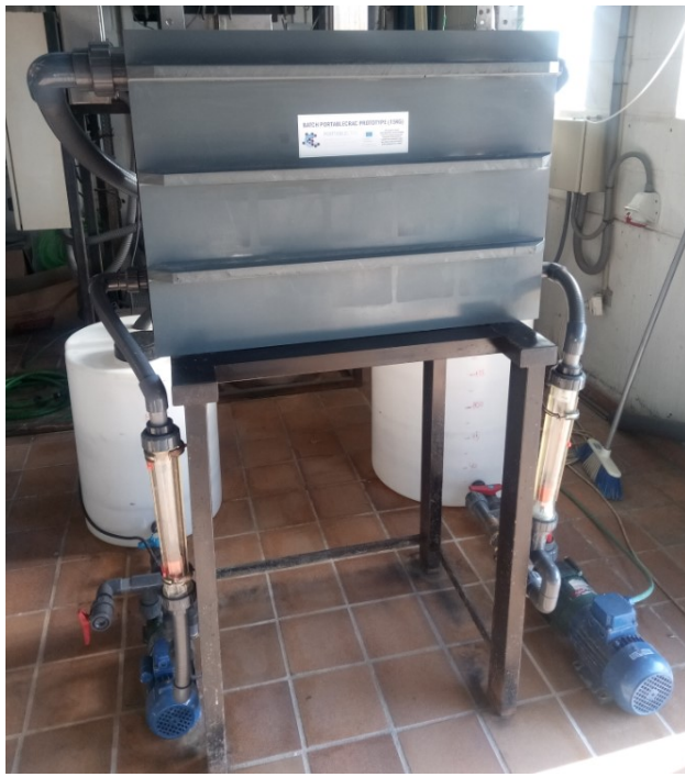
Picture 1: electrochemical reactor front view in parallel plane electrode configuration -15 kg. treatment capacity-
