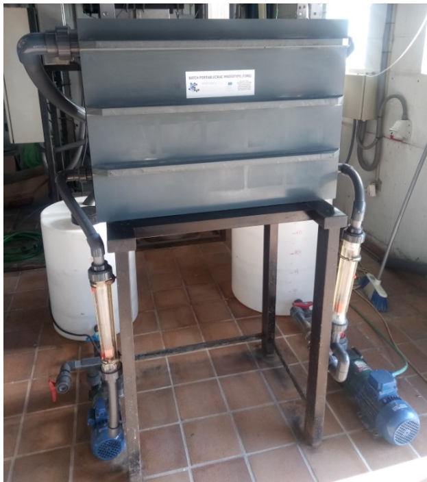
Picture 1: electrochemical reactor front view in parallel plane electrode configuration -15 kg. treatment capacity-
