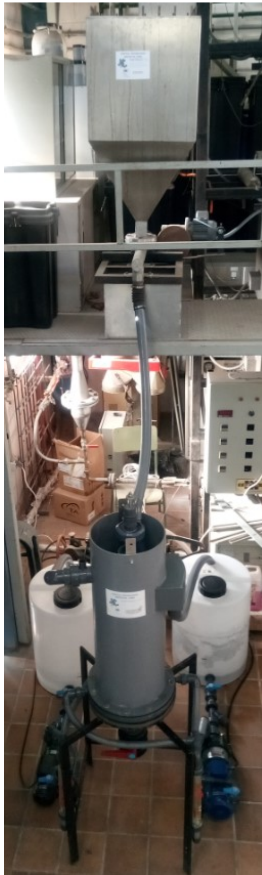
Picture 2: electrochemical reactor front view in concentric cylindrical electrode configuration -10 kg. treatment capacity-
