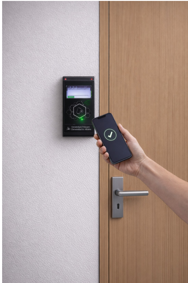
Fig. 1. Installed reader device
