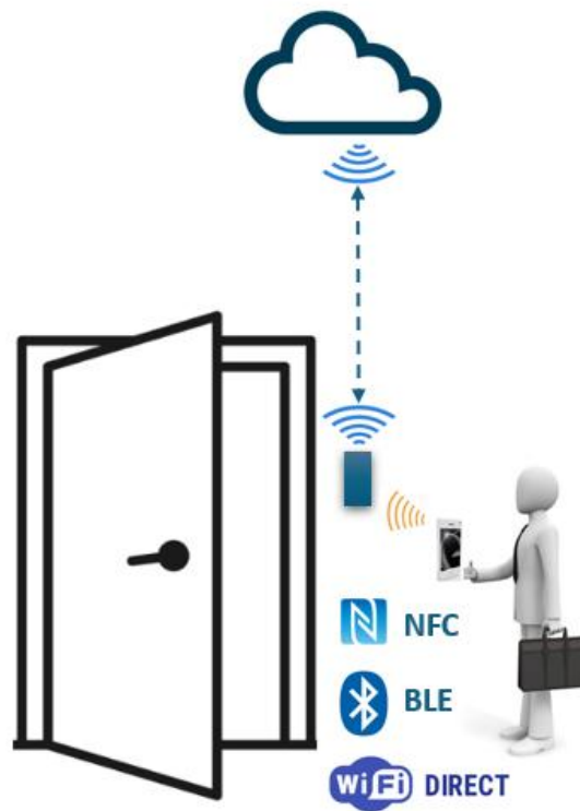
Fig 3. IoT architecture for distributed access control
