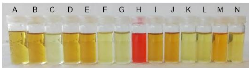
Figure 2: Nitrite ion selective detection test ( \text{NaNO}_2 , reddish solution), against thirteen anions, using a formylindolizine in acidic medium. Salts: \text{KCN} , \text{PhCO}_2\text{K} , \text{KF} , \text{KCl} , \text{KBr} , \text{KI} , \text{KOAc} , \text{K}_2\text{P}_4\text{O}_7 , \text{K}_3\text{PO}_4 , \text{KH}_2\text{PO}_4 , \text{NaN}_3 , \text{K}_2\text{S} y \text{NaHS} . All concentrations are 10^{-4} M.
