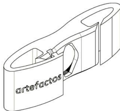
Figure 1: Perspective view of the device where you can see the different parts that make it up (central body, closing side, free opening side and housing for personal aid accessories).
