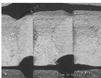
Figure 2: photograph taken by SEM microscopy showing the homogeneous distribution of the powder catalyst on the channel walls of a polymeric monolith.
