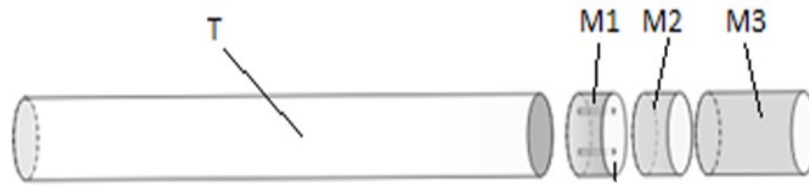
Figure 1: tobacco column (T) and combined filter formed by: the primary membrane (M1), the intermediate membrane (M2) and the outer membrane (M3).
