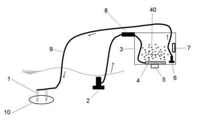
Figure 1. Diagram of the injection system, showing all the elements involved in the anoxic marine sediment remediation procedure. 1) Nozzles; 2) Suction pump; 3) Tank; 4) Diffusers; 5) Air blower; 6) Drive pump; 7) Oximeter; 8) Filters; 9) Pipelines; 10) Sediment to treat; 40) Small bubbles.
