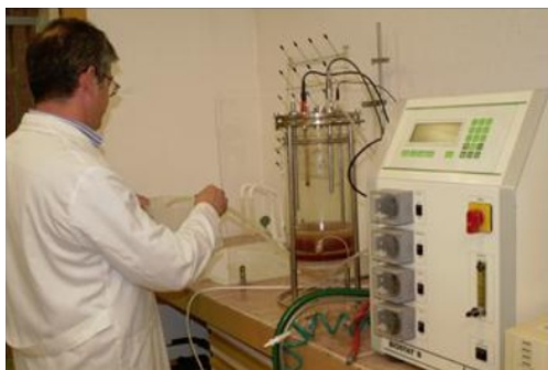
Figure 6: Emptying operation of the bioreactor.
