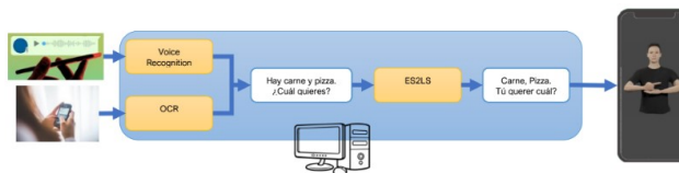
Figure 2. Diagram of the functionality corresponding to the generation of the signing by means of a virtual avatar from text or audio entered by a user.
