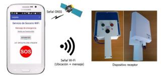
The **smartphone** must be equipped with a GNSS receiver and a Wi-Fi interface, elements found in almost all smartphones on the market. In addition, it must have installed an App, specifically designed by the researchers of the University, that emits the distress signal detectable by the receiving device. The developed App can be used by any smartphone that owns the Android operating system. Also, the App could be developed for other operating systems.
