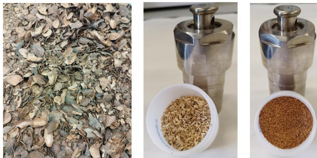
Picture 2: Different biomass residues used in the laboratory tests, including cocoa shells, eucalyptus wood and almond shells, respectively.
