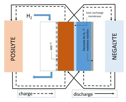
[1] GDE: Gas diffusion electrode [2] Electrode catalysed using an appropriate metal.
