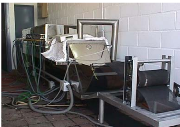
Figure 4. Pilot plant for the manufacture of activated carbon cloth.
