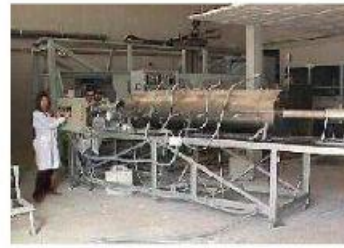
Figure 2. Rotary furnace pilot plant.
