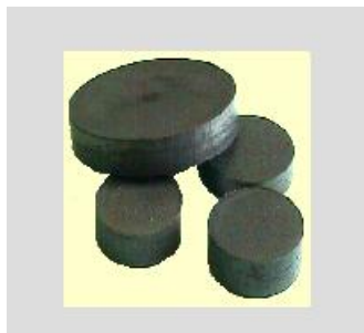
Figure 3. Solid monoliths of activated carbon
