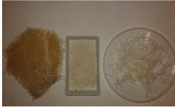
Left: Fiber-resin composite material before fiber recovery treatment. Right: Fiberglass recovered after chemical treatment. Center: degraded resin residue after the chemical treatment.
