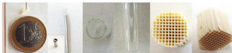
Figure 1. Selected materials, from left to right: Fused silica capillary (i.d. 0.25 mm), stainless steel tubing (i.d. 1.6 mm), glass tube (i.d. 7.6 mm), and multichannel cordierite monolith (i.d.channel 1.2 mm).
