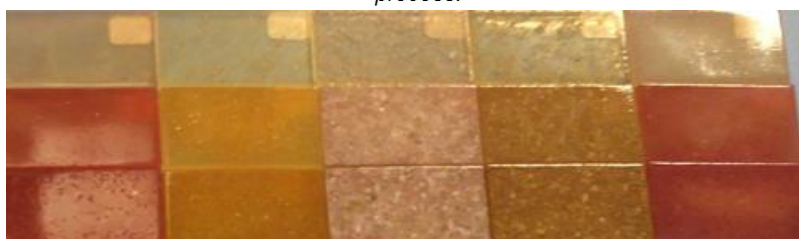
Figure 3. Epoxy bioresin nanocomposites, with \beta -carotene nanopigments, from different synthesis process.
