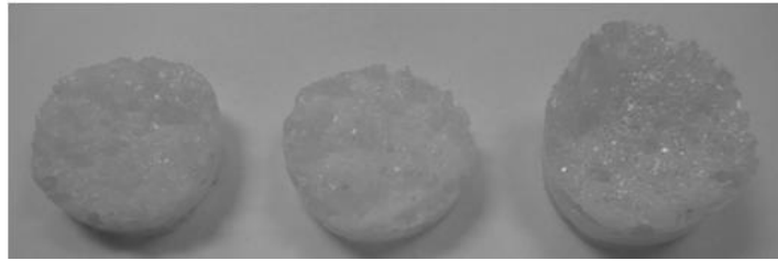
Some polyurethane foams with different extent of foaming produced by using different formulations.
