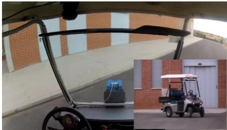
Figure 1. Autonomous golf cart circulating on the University of Alicante
