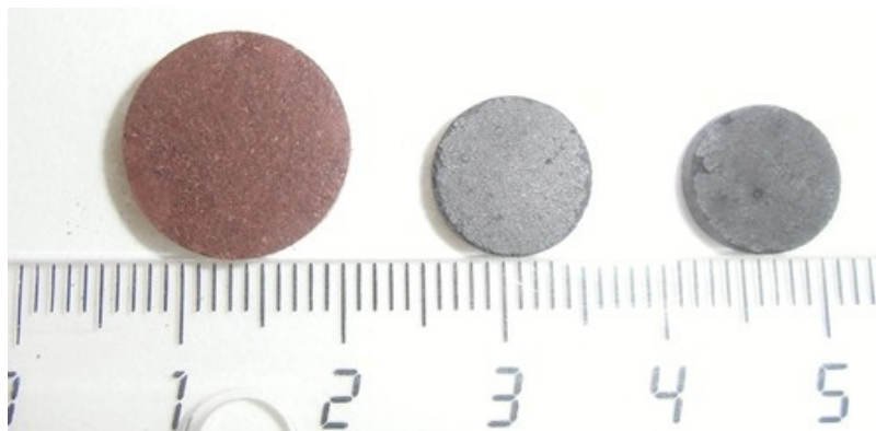
Figure 1: Activated carbon monolith obtained from cocoa shell during the three different steps (from left to right): mounding, carbonized and activated
