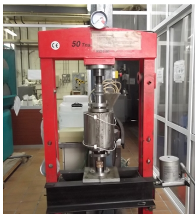
Figure 3.- Hydraulic piston press briquette machine used
