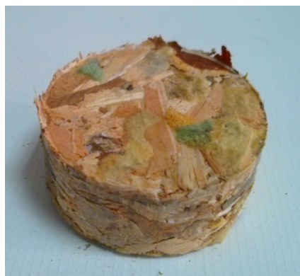
Figure 2.- Briquette obtained with a mixture of furniture waste and polyurethane foam
