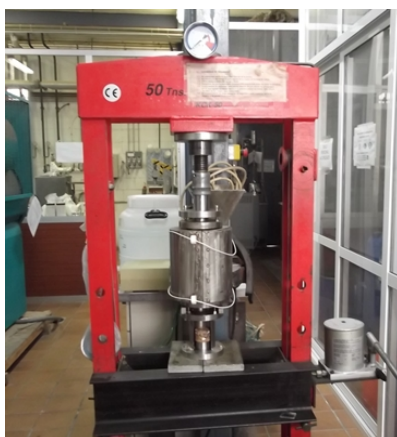
Figure 3.- Hydraulic piston press briquette machine used
