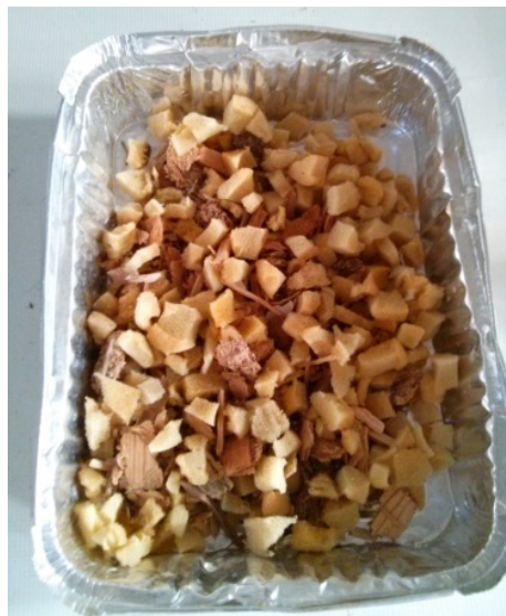
Figure 1.- Initial mixture of furniture waste with polyurethane foam
