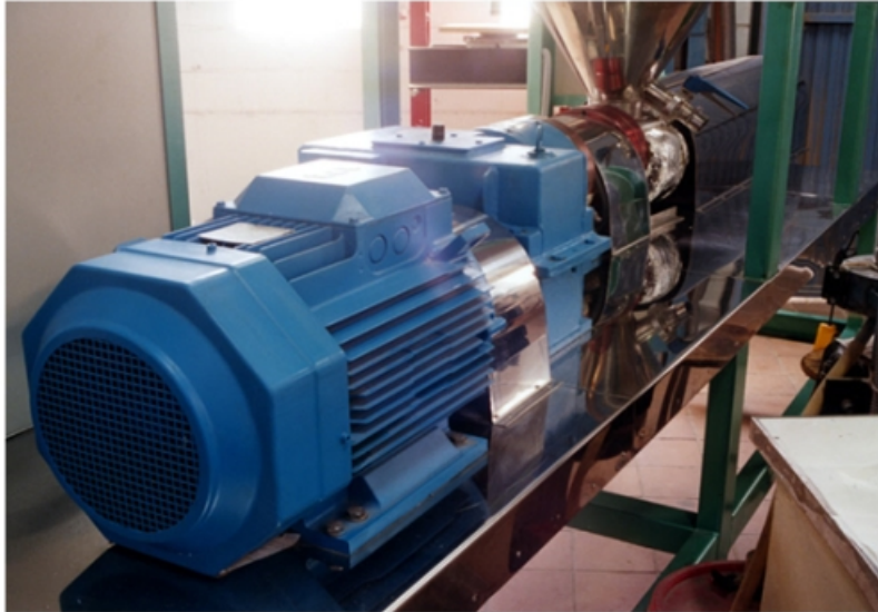
Engine + Reductor and axial box
